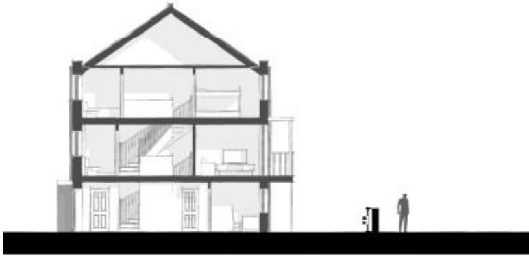
Plot section of the previous proposal, showing a 1.1m high boundary fence and flat topography.
