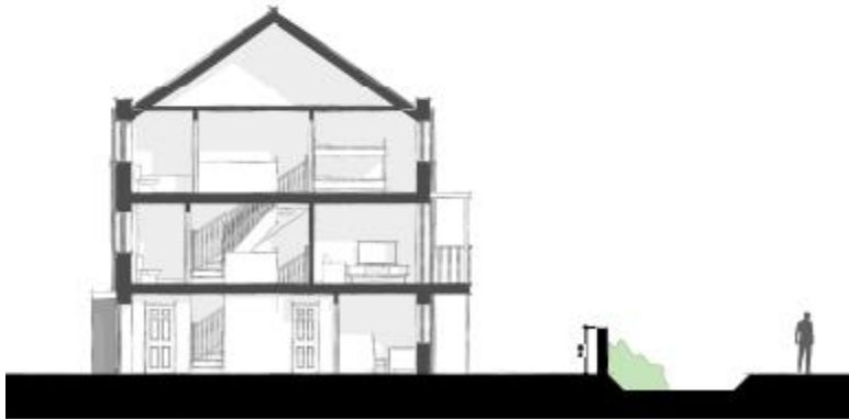
Plot section of the new proposal, showing a 1.4m high boundary fence, additional slopes and spiked hedging. The depression in the ground is intended to be 0.4m, giving an overall boundary height on 1.8m. We believe this combination will deter any persons looking to access the private gardens.
